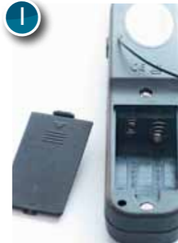
1 Insert two AA batteries into the holder. To operate, press the button on the side. A red light indicates that the tool is ready to use.
