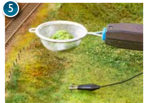
5 Shake the applicator, switch it on and gently move it from side to side about 3cm to 4cm over the surface of the glue.
