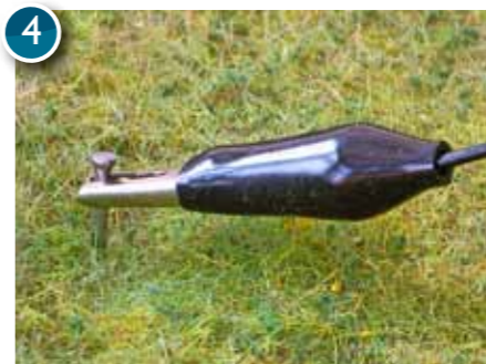
4 Hammer the supplied nail into the baseboard where you intend to plant and attach the crocodile clip to it. Alternatively, earth the applicator on a piece of nearby track.
