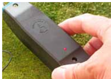
Press the button on the side and the red light shows that DoubleO's applicator is ready to use.
